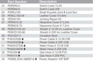
\*Note: Power cable, gas and water hose assemblies are configured by utilizing the main part number and a termination suffix from the appropriate termination table on page 10.
